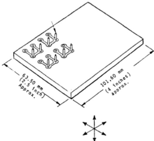
NOTE: Printed Wiring Board to be rigidly mounted along four edges.
