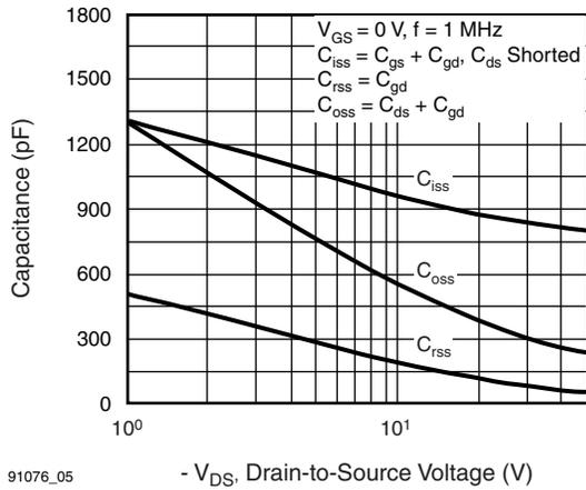
Fig. 5 - Typical Capacitance vs. Drain-to-Source Voltage
