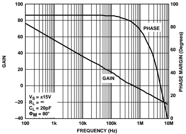
Figure 22. Open-Loop Gain and Phase vs. Frequency
