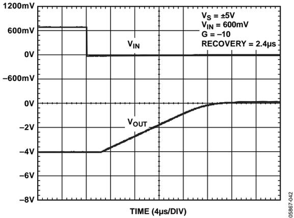
Figure 38. Positive Overload Recovery
