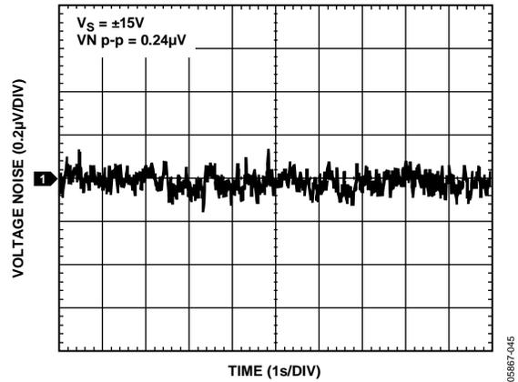
Figure 41. Voltage Noise (0.1 Hz to 10 Hz)
