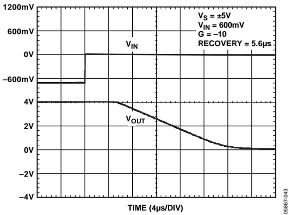
Figure 39. Negative Overload Recovery
