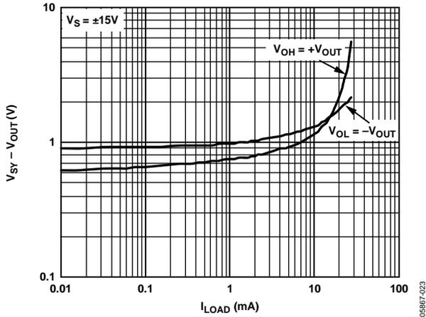
Figure 20. Output Voltage Swing vs. Load Current
