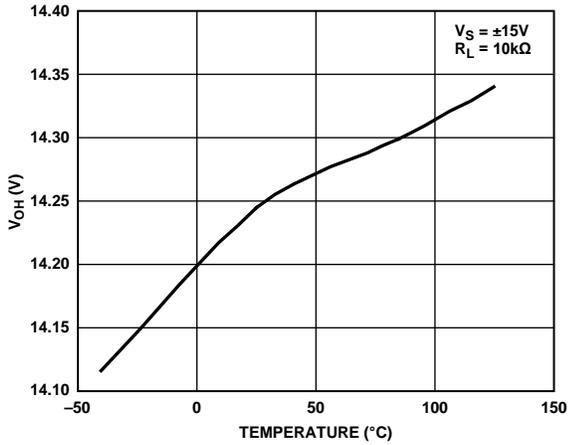
Figure 9. Positive Output Voltage Swing vs. Temperature
