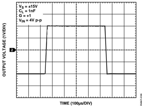
Figure 34. Large-Signal Transient
