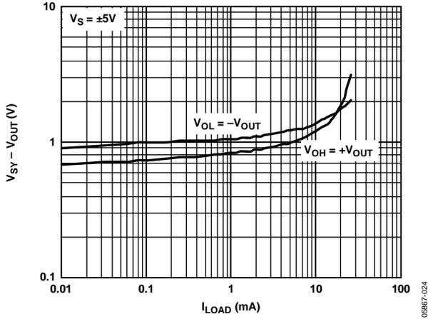
Figure 21. Output Voltage Swing vs. Load Current
