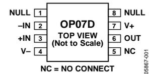
Figure 1. 8-Lead SOIC\_N (R-8), 8-Lead DIP (N-8)
