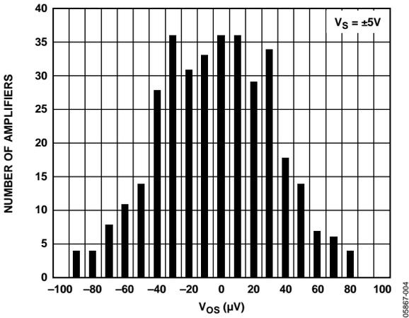
Figure 3. Number of Amplifiers vs. Offset Voltage
