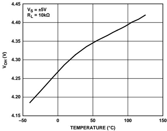
Figure 10. Positive Output Voltage Swing vs. Temperature
