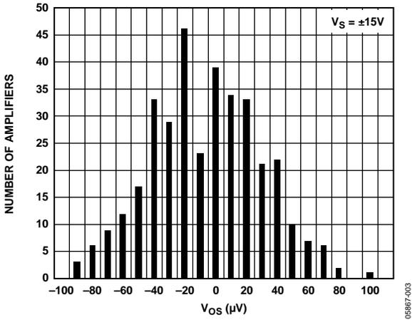
Figure 2. Number of Amplifiers vs. Offset Voltage
