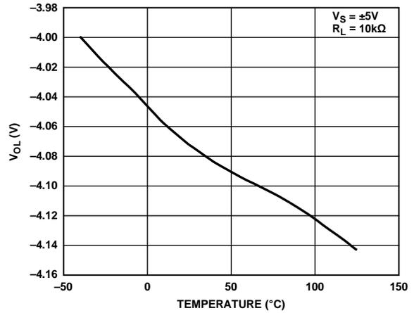
Figure 12. Negative Output Voltage Swing vs. Temperature
