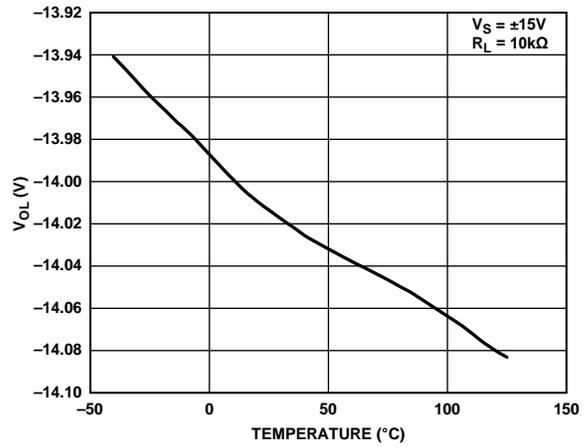
Figure 11. Negative Output Voltage Swing vs. Temperature
