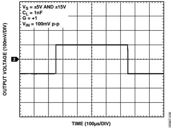
Figure 33. Small-Signal Transient
