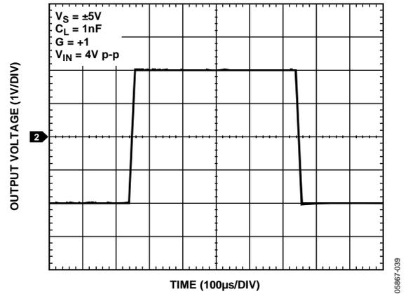
Figure 35. Large-Signal Transient
