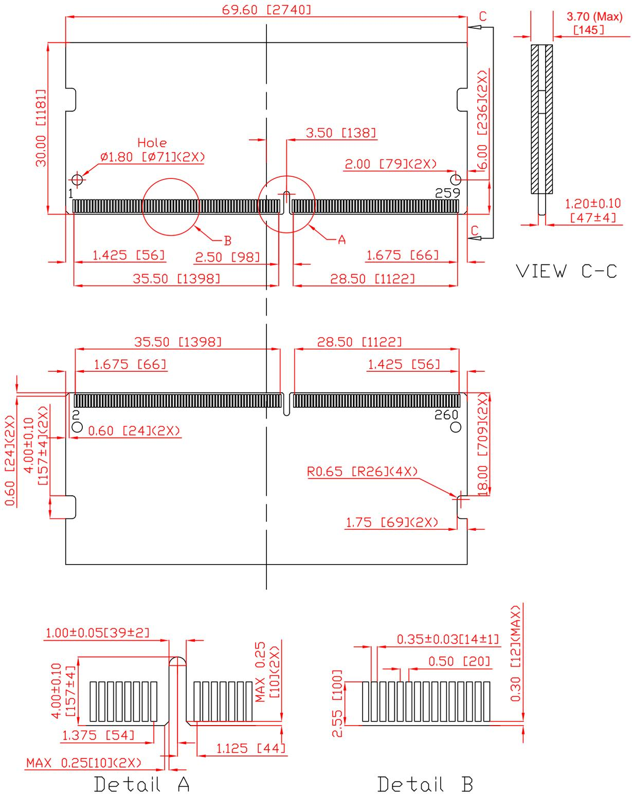
(All dimensions are in millimeters with  $\pm 0.15$ mm tolerance unless specified otherwise.)
