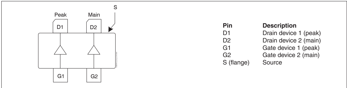
Lead connections for PTAC260302FC
