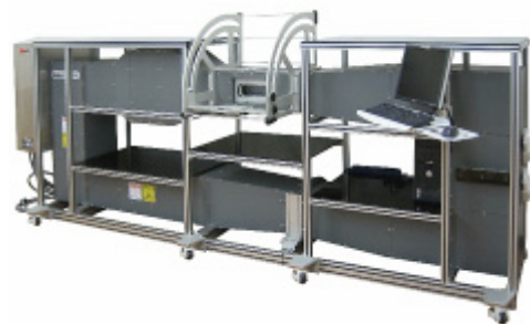
Fig. D: FDK Original Wind Tunnel
