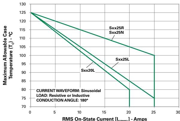
**Figure 8: Maximum Allowable Ambient Temperature vs. RMS On-State Current**
