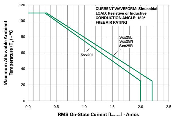
**Figure 9: Maximum Allowable Ambient Temperature vs. Average On-State Current**
