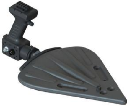
Alaris direction-finding smart antenna.
