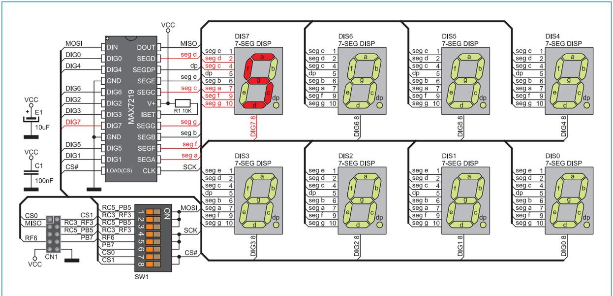
Figure 4: Time-division multiplexing performed on the DIS7 display
