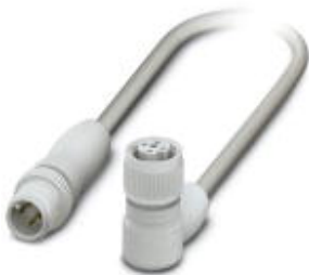
Sensor/Actuator cable, 4-position, PP-EPDM halogen-free, Gray RAL 7035, Plug straight M12, A-coded, on Socket angled M12, A-coded, with 3 LEDs, Cable length: 0.3 m, Hygienic design, with plastic knurl
