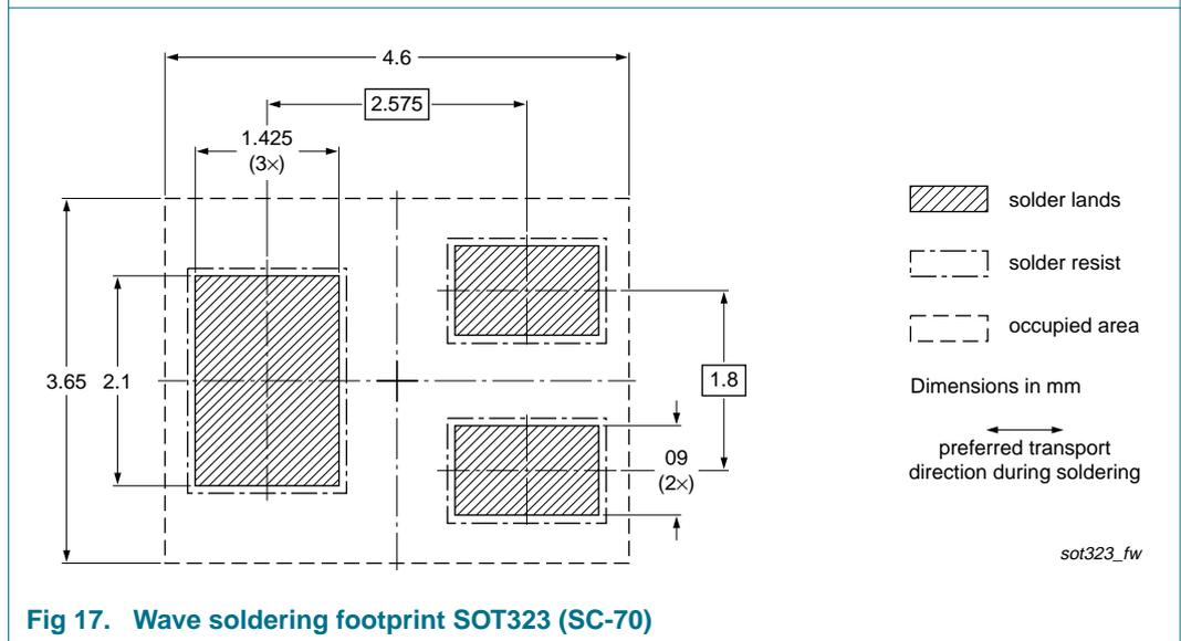
**Fig 17. Wave soldering footprint SOT323 (SC-70)**
