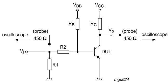
$I_C = -0.5\text{ A}$ ;  $I_{Bon} = -25\text{ mA}$ ;  $I_{Boff} = 25\text{ mA}$ ;  $R_1 = \text{open}$ ;  $R_2 = 100\ \Omega$ ;  $R_B = 300\ \Omega$ ;  $R_C = 20\ \Omega$
