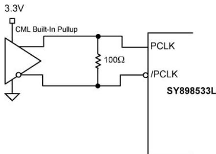
**Figure 3b. CML Built-in Pull-up
