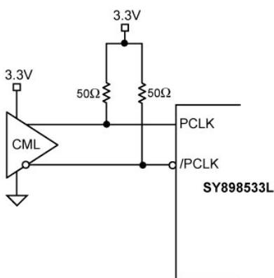
**Figure 3a. CML Open Collector Interface
