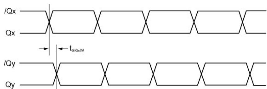
Figure 1c. Output-to-Output Skew
