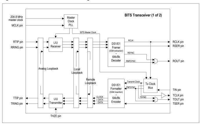
**Note:** The ZL81000 BITS transceivers are full-featured DS1/E1 LIUs and framers. To keep configuration as simple as possible, only the features most commonly used for clock synchronization applications are made visible in this data sheet. If your application requires LIU or framer features not described in this document, contact Microsemi timing products technical support for additional information.
