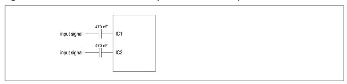
For input CC signals compliant with Telcordia GR-378 (amplitude 2.7V to 5.5V) or ITU G.703 Section 4.2.2 option b)  $(3V\pm0.5V)$ , the signal should be attenuated by a factor of 3 (or more) before being presented to IC1A or IC2A. Input CC signals with a 1V nominal pulse amplitude can be presented unattenuated.
