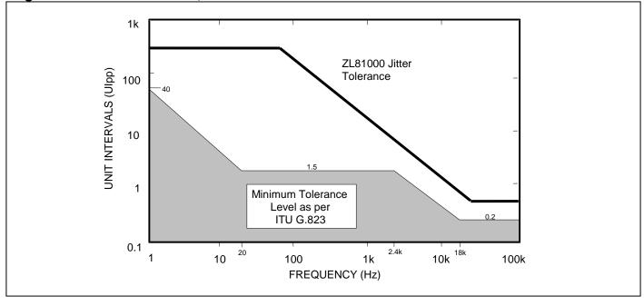
Figure 6-7. Jitter Tolerance, E1 and 2048kHz Modes
