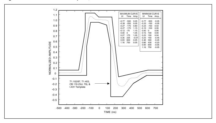
Figure 6-9. Transmit Pulse Template, E1 Mode
