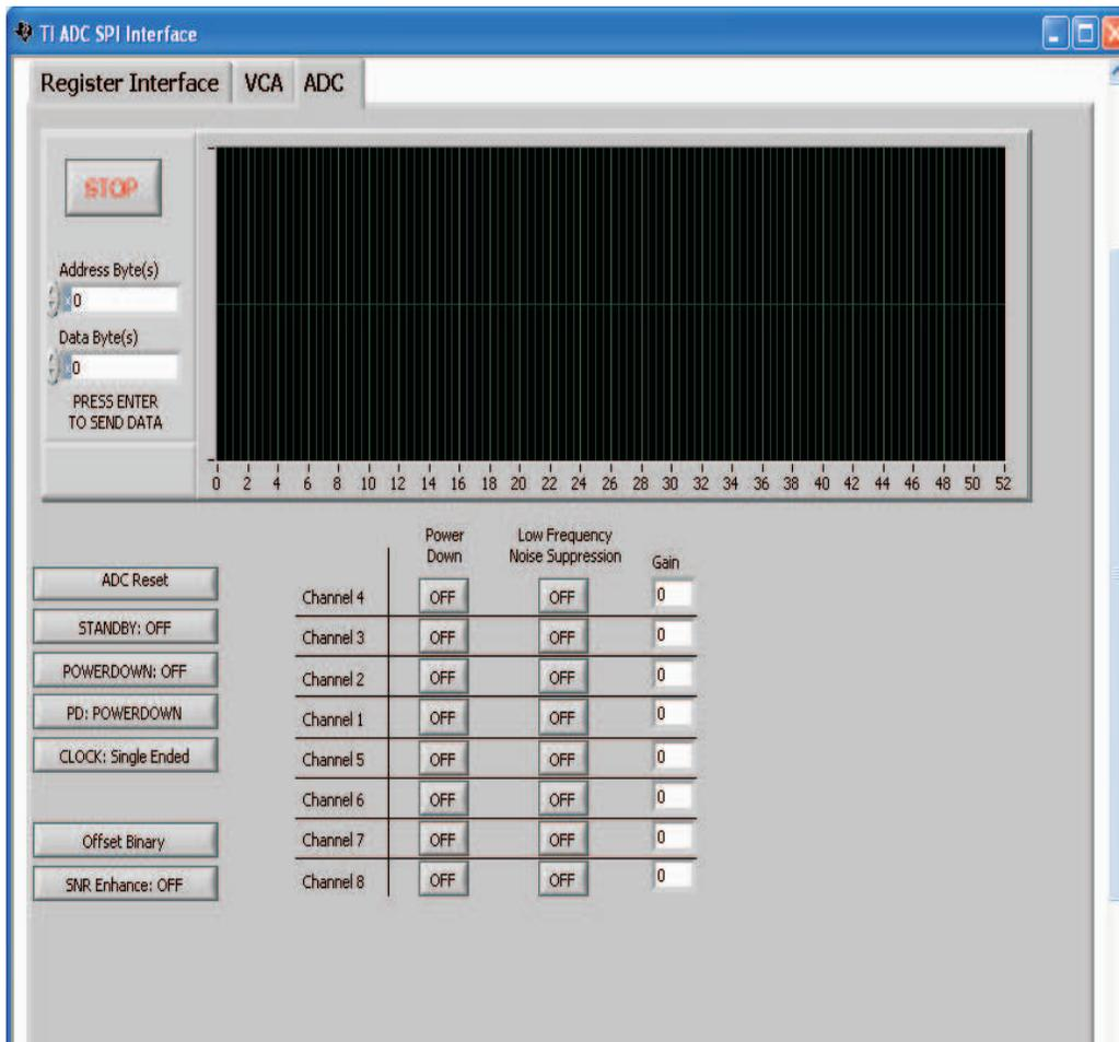
Figure 7. AFE5804EVM USB SPI Interface for ADC Setup
