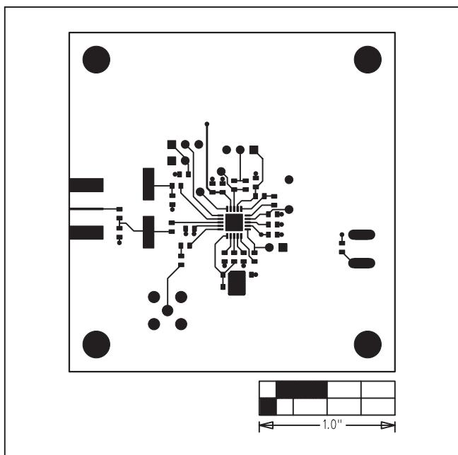
Figure 4. MAX7036 EV Kit PCB Layout—Component Side
