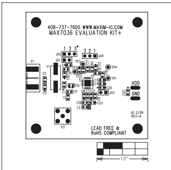
Figure 3. MAX7036 EV Kit Component Placement Guide—Component Side
