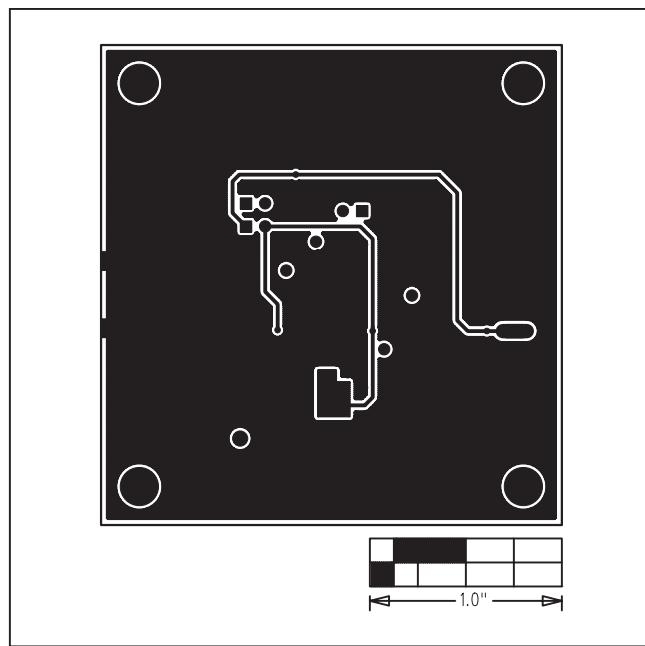
Figure 5. MAX7036 EV Kit PCB Layout—Solder Side
