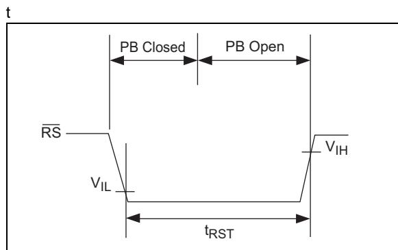
**FIGURE 3-2:**  $\overline{RS}$  Pulled Low By Push-Button Reset
