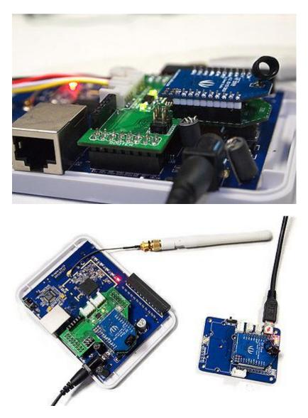
There are two RFbees used in this demo. One was inserted onto the Dragrove's XBee socket and
