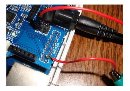
This solution forces COLD to LOW, which then allows the board to boot. You have to keep the COLD pin LOW to prevent Dragino from rebooting. Once the Dragino boots, you can program the daughter board (as described in the wiki further below) to bring COLD to LOW at startup.
