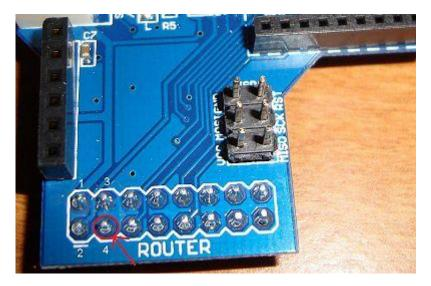
The solution is to link a wire between COLD pin and Ground as shown in the image below:
