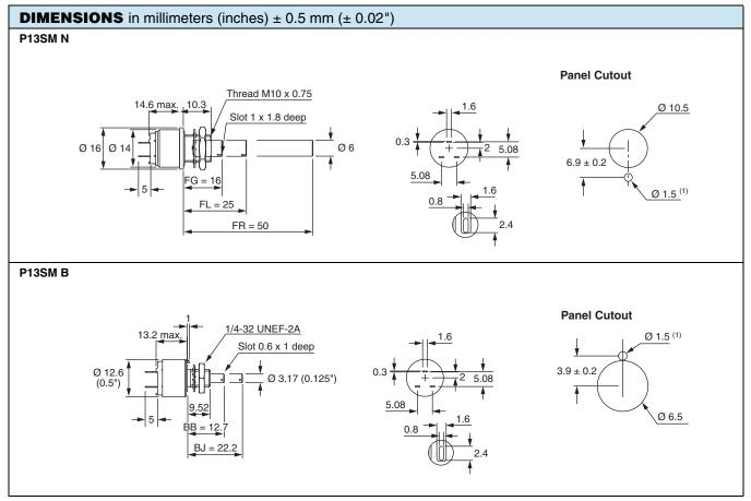
(1) CAUTION: Ø 1.5 of panel cut out must not be fully through hole.
