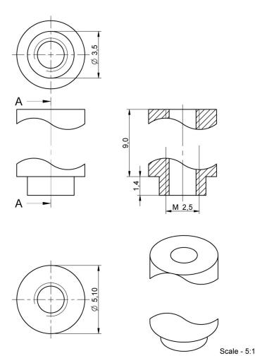
Technical Tolerances according to DIN ISO 2768m
