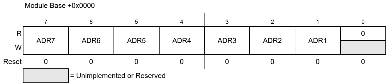
Figure 16-3. IIC Bus Address Register (IBAD)
