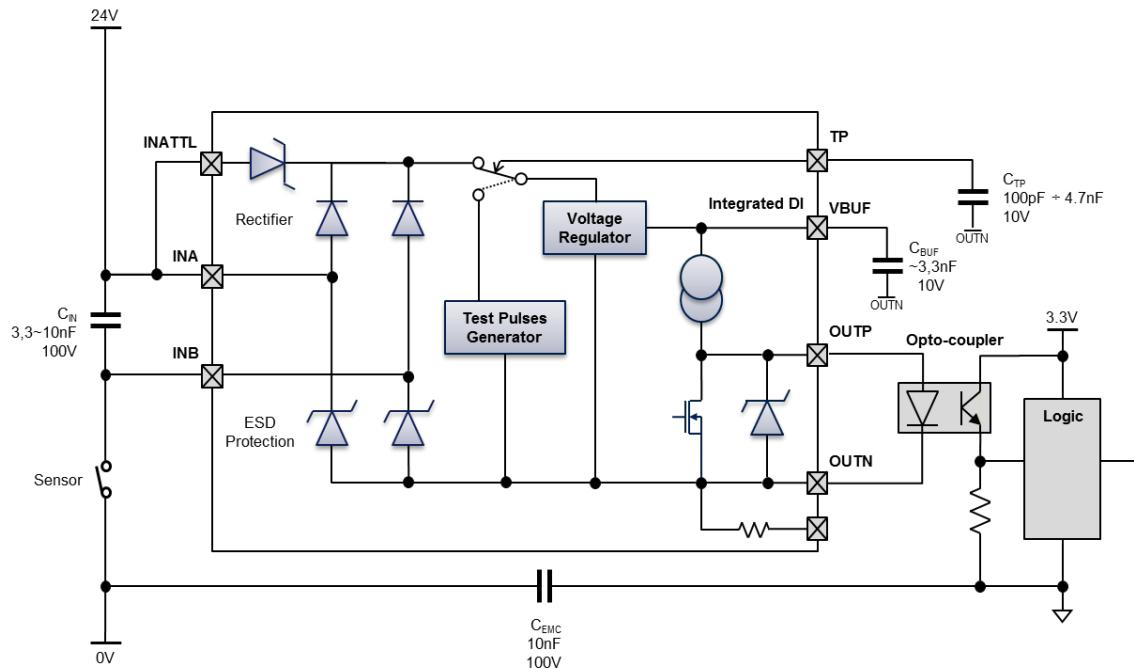
Figure 11. High side – non-isolated configuration
