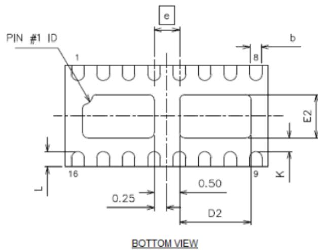
**Table 7.** QFN 2X4-16L package mechanical data
