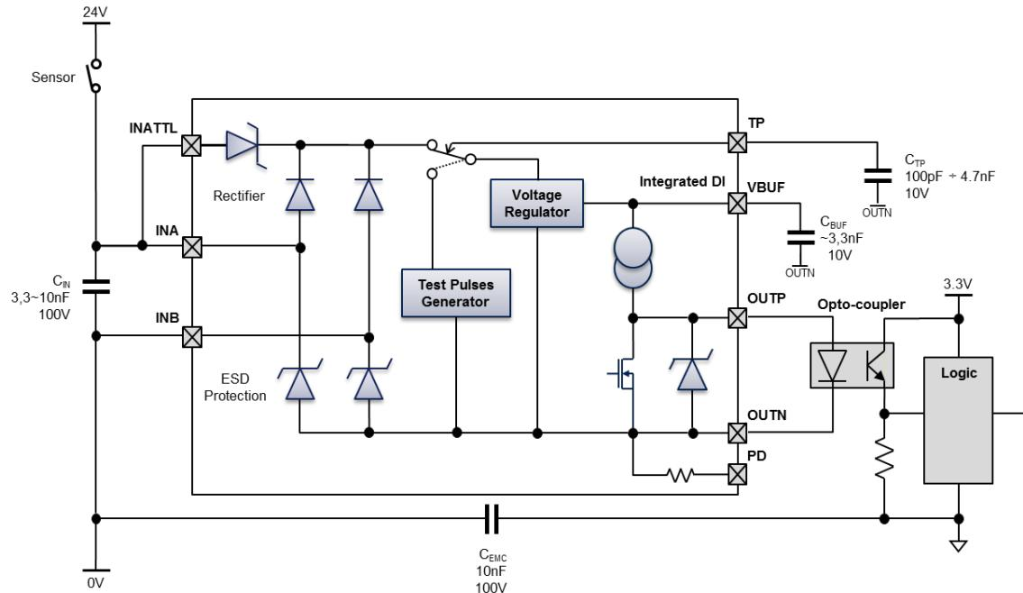
Figure 10. Low side – isolated configuration
