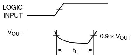
Figure 4. Break Before Make Interval Timing
