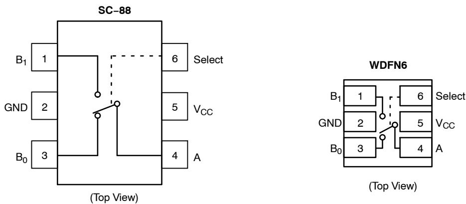
Figure 1. Pin Assignment &amp; Logic Diagram
