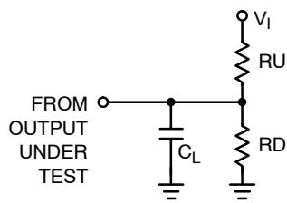
Figure 2. AC Test Circuit
