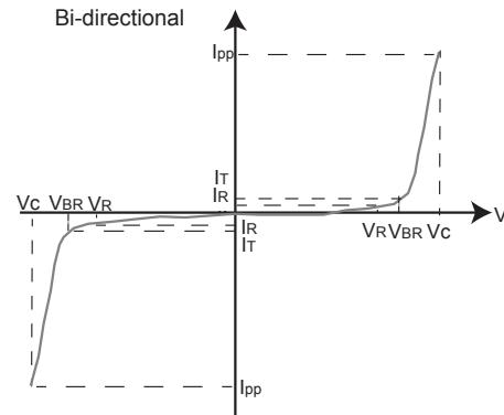
**P<sub>PPM</sub>** **Peak Pulse Power Dissipation** – Max power dissipation
