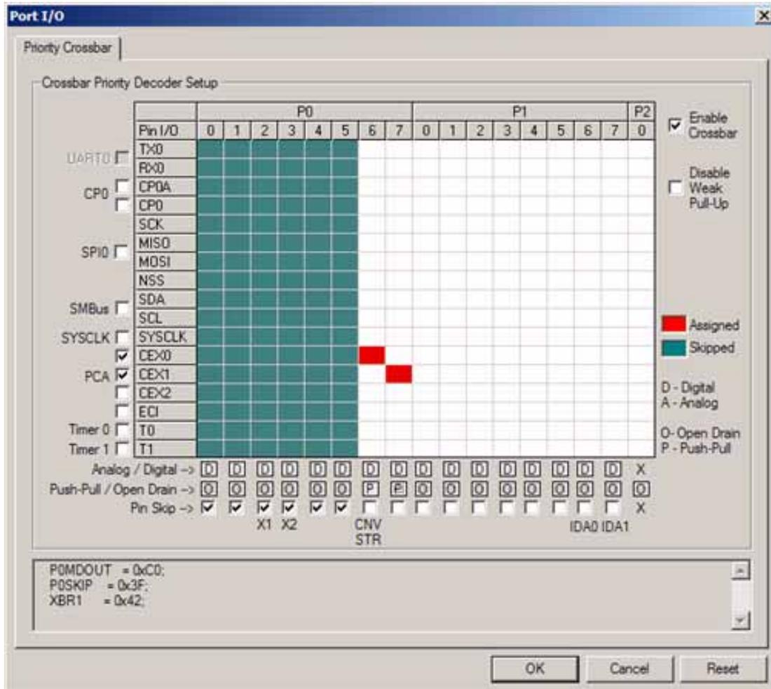
Figure 14. Peripheral Configuration Wizard - Port I/O Window
