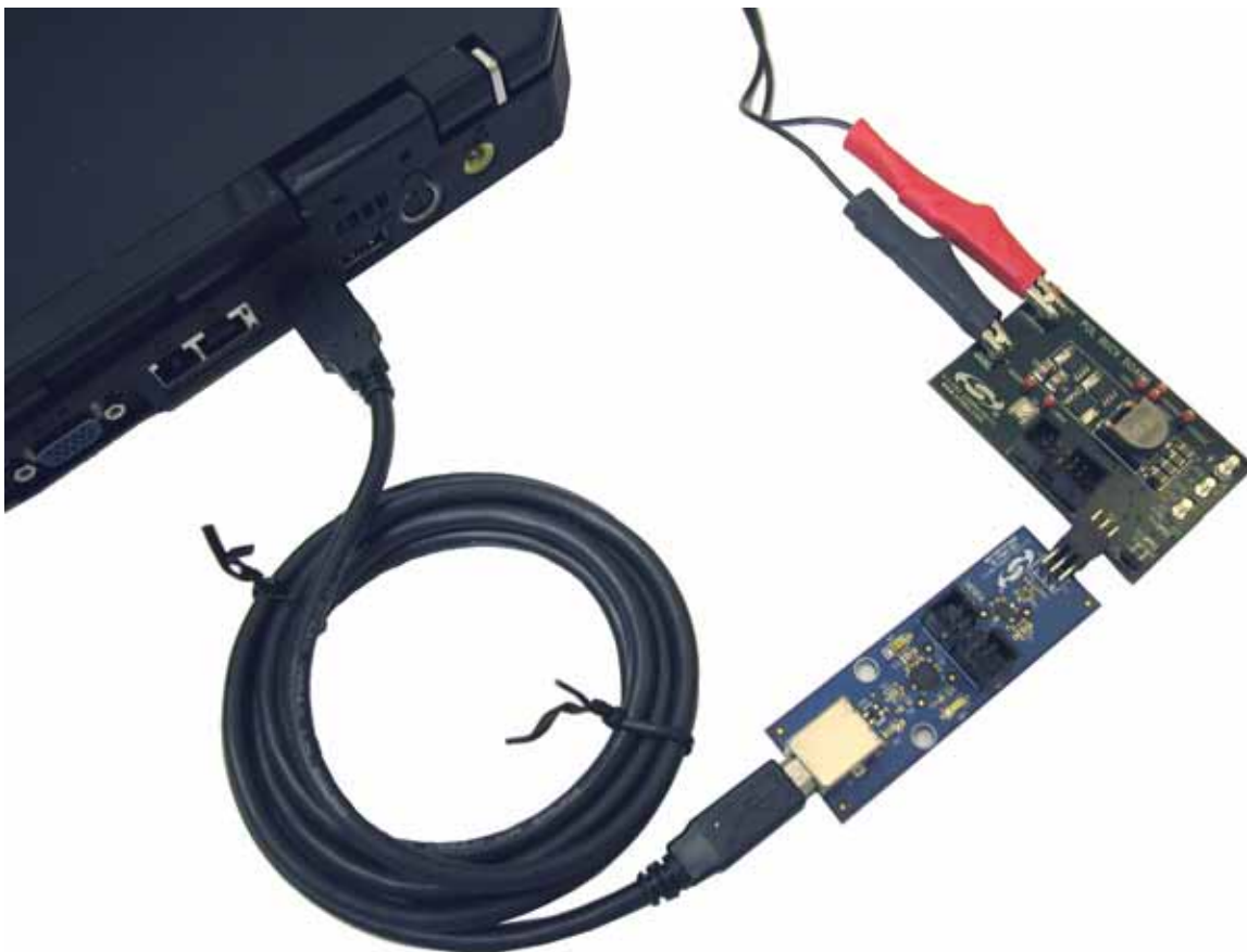
Figure 4. USB to SMBus Bridge Board Connection (Load not Connected)
