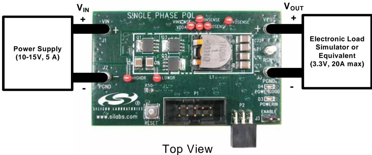
Figure 2. Board Power Configuration
