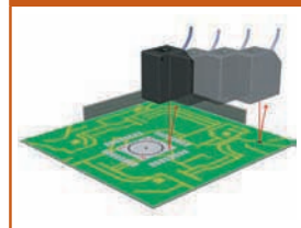
Inspecting Board Heights
