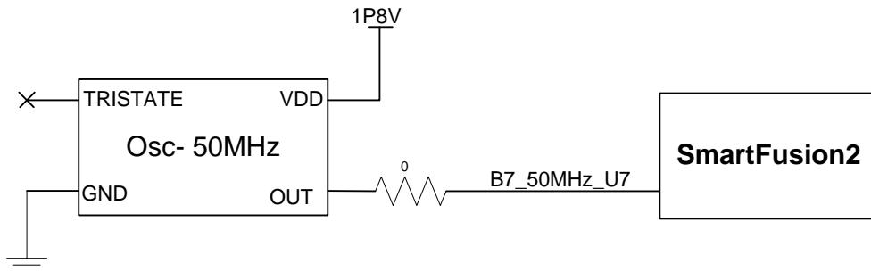
**Figure 15 - 50 MHz - Clock Oscillator Interface**
