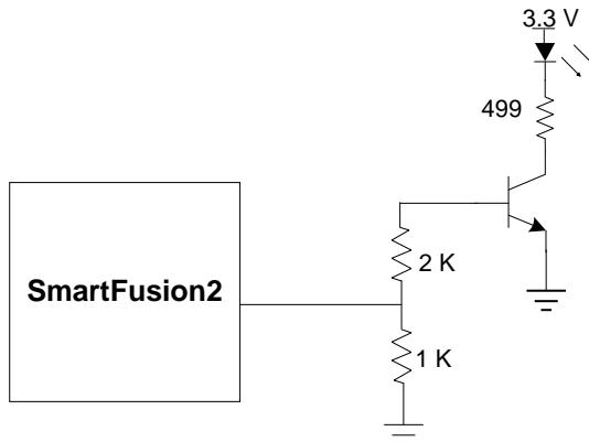
**Figure 17 · LEDs Interface**
