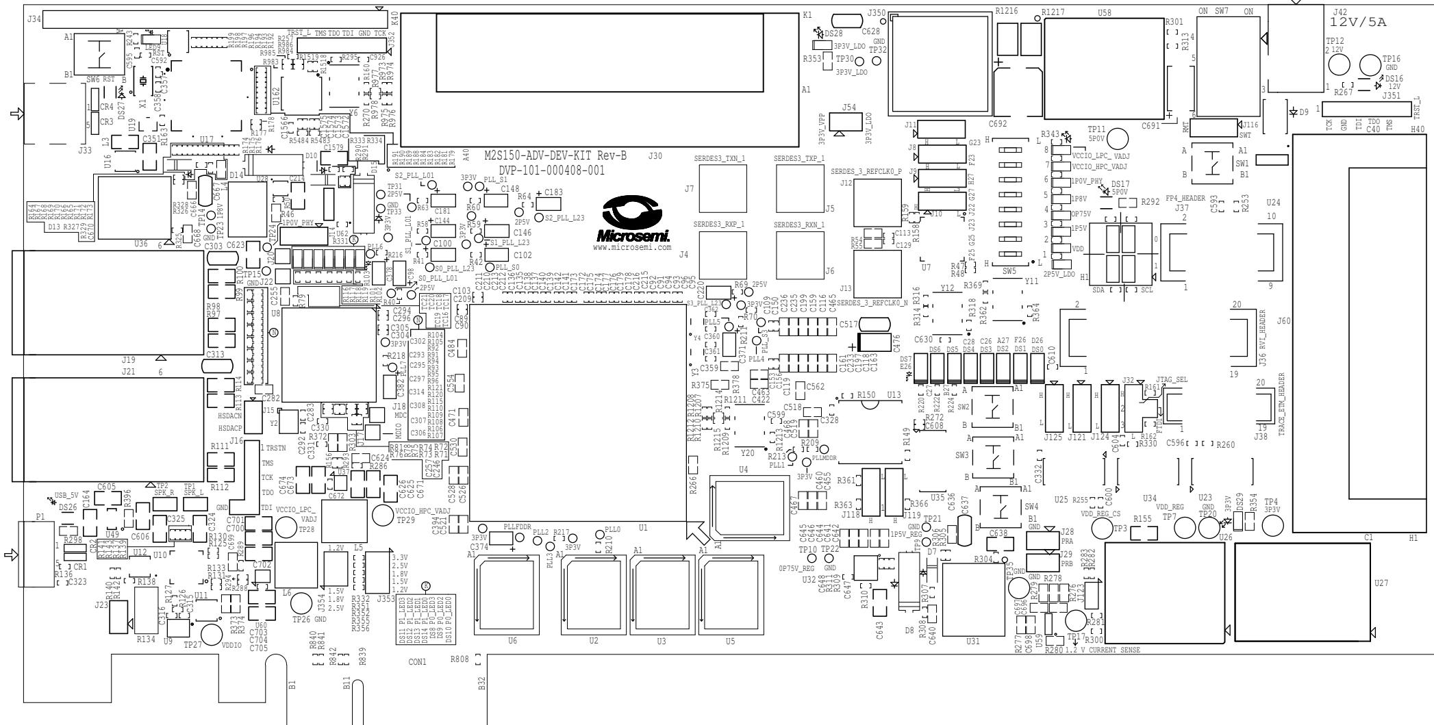
Figure 20 · SmartFusion2 Advanced Development Kit Board Silkscreen Top View
