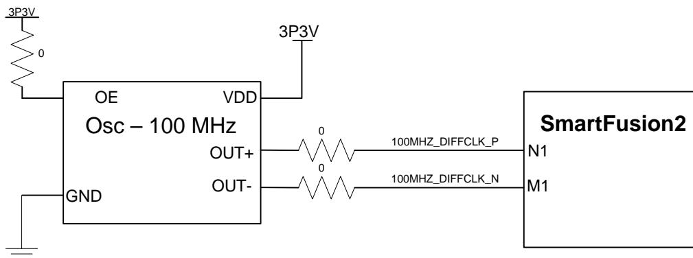
**Figure 16 - 100 MHz - Clock Oscillator Interface**
