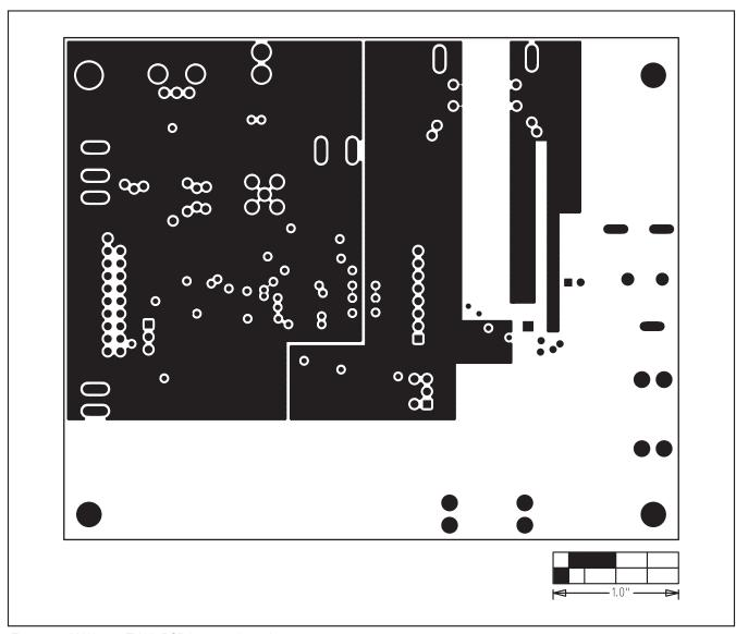
Figure 19. MAX9850 EV Kit PCB Layout—Inner Layer 3
