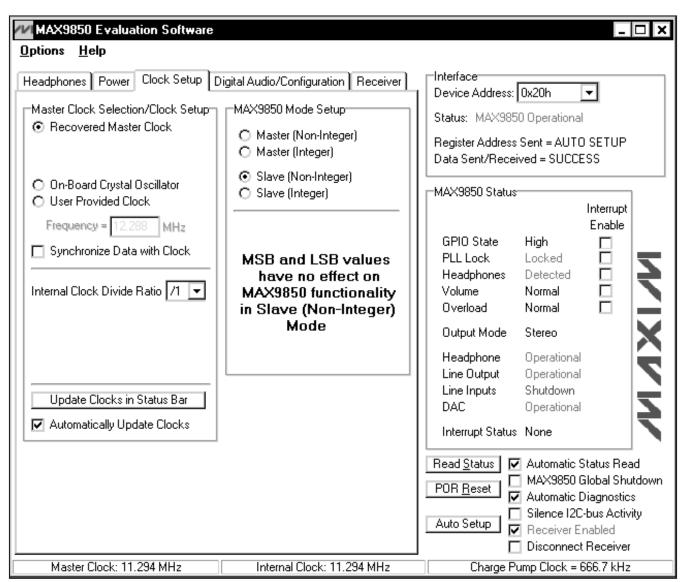
Figure 5. MAX9850 EV Kit Software Clock Setup Tab
