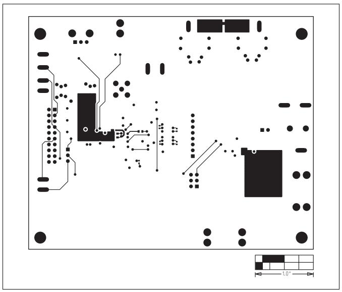
Figure 20. MAX9850 EV Kit PCB Layout—Solder Side
