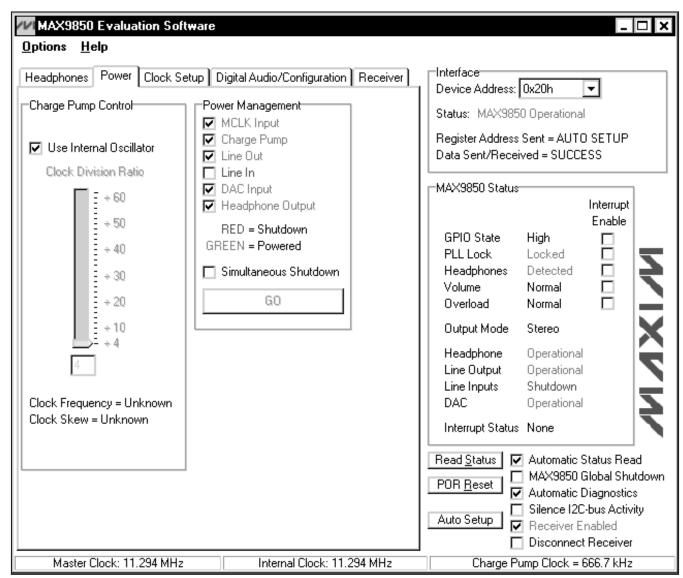
Figure 4. MAX9850 EV Kit Software Power Tab
