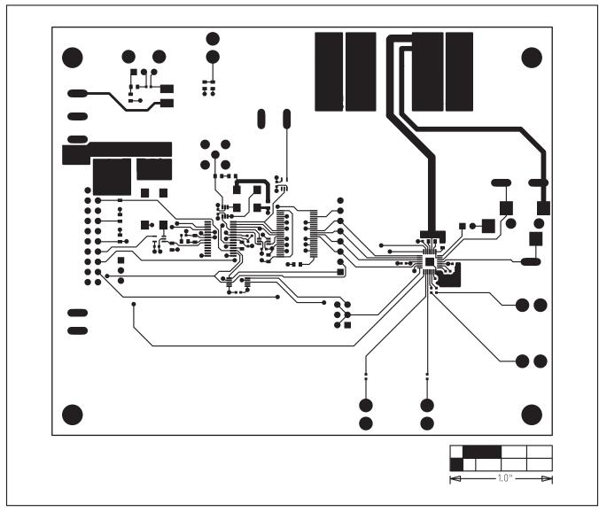
Figure 17. MAX9850 EV Kit PCB Layout—Component Side
