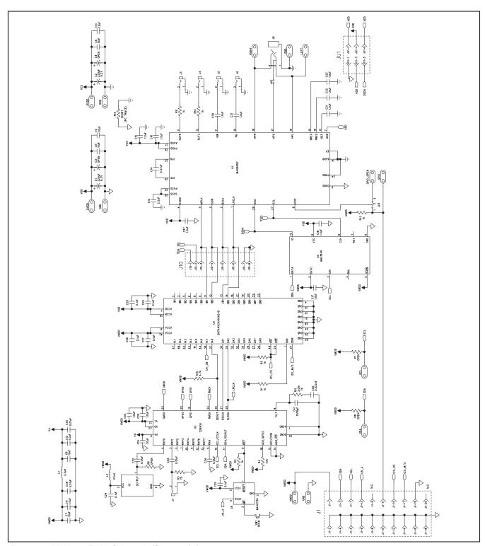
Figure 15a. MAX9850 EV Kit Schematic (Sheet 1 of 2)
