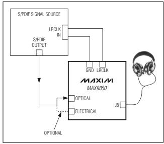
Figure 14. Synchronized MAX9850 EV Kit Diagram
