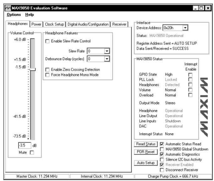
Figure 1. MAX9850 EV Kit Software Main Window
