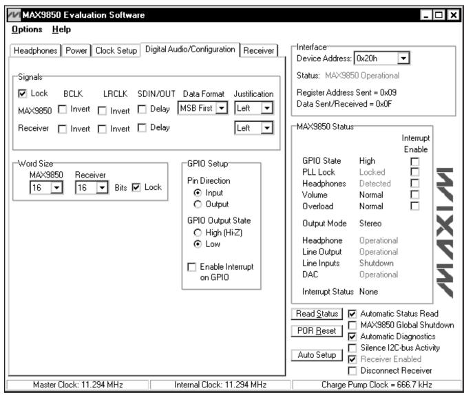
Figure 10. MAX9850 EV Kit Software Digital Audio/Configuration Tab
