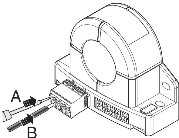
Figure 5 Spring-cage connection
