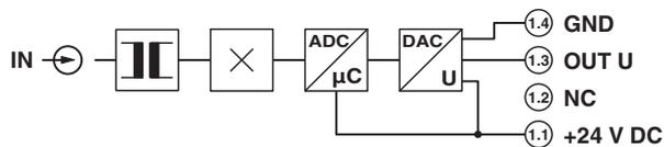
Figure 2 Block diagram for voltage output
