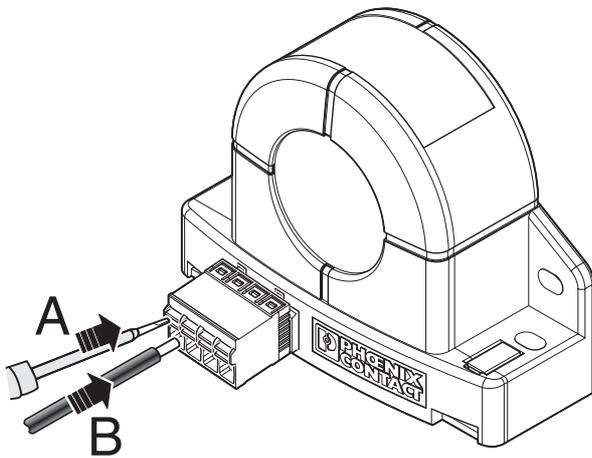
Figure 5 Spring-cage connection
