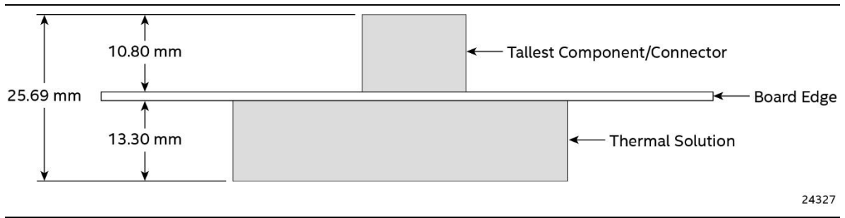
Figure 18. Board Height Dimensions
