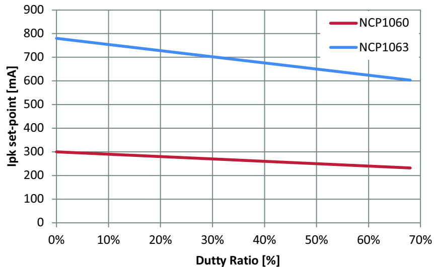
Figure 43. I_{PK} set-point varies with power switch on time, which is caused by the ramp compensation.
