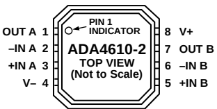
Figure 5. ADA4610-2 Pin Configuration, 8-Lead LFCSP_VD (CP Suffix)
