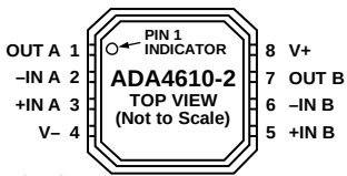
Figure 5. ADA4610-2 Pin Configuration, 8-Lead LFCSP_VD (CP Suffix)
