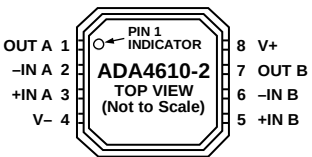
Figure 5. ADA4610-2 Pin Configuration, 8-Lead LFCSP_VD (CP Suffix)
