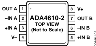
Figure 4. ADA4610-2 Pin Configuration, 8-Lead MSOP (RM Suffix)
