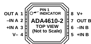
Figure 5. ADA4610-2 Pin Configuration, 8-Lead LFCSP_VD (CP Suffix)
