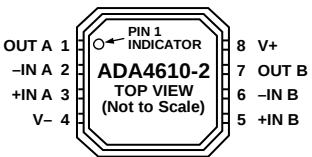
Figure 5. ADA4610-2 Pin Configuration, 8-Lead LFCSP_VD (CP Suffix)
