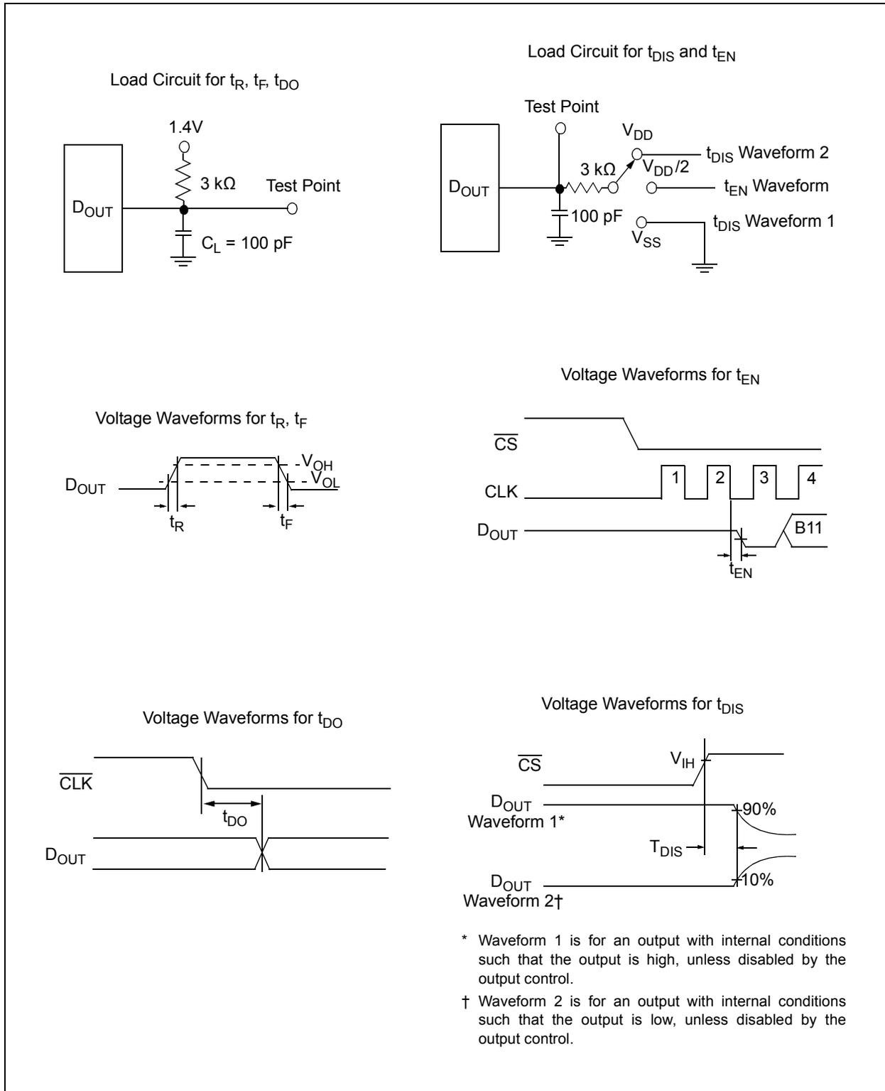
**FIGURE 1-2:** Test Circuits.
