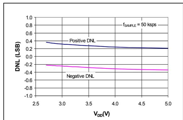
**FIGURE 2-12:** Differential Nonlinearity (DNL) vs.  $V_{DD}$ .
