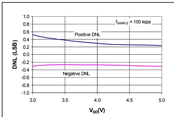
**FIGURE 2-9:** Differential Nonlinearity (DNL) vs.  $V_{DD}$ .
