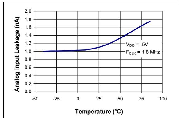
**FIGURE 2-36:** Analog Input leakage current vs. Temperature.
