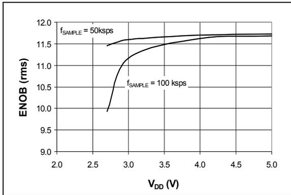
**FIGURE 2-25:** Effective Number of Bits (ENOB) vs.  $V_{DD}$ .
