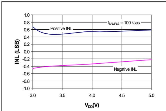
**FIGURE 2-2:** Integral Nonlinearity (INL) vs.  $V_{DD}$ .
