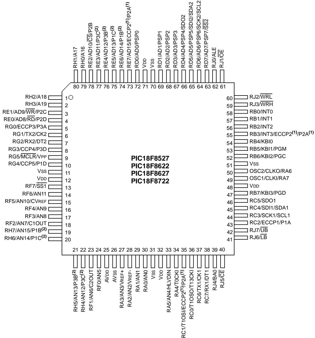
**Note** 1: The ECCP2/P2A pin placement is determined by the CCP2MX Configuration bit and Processor mode settings.
