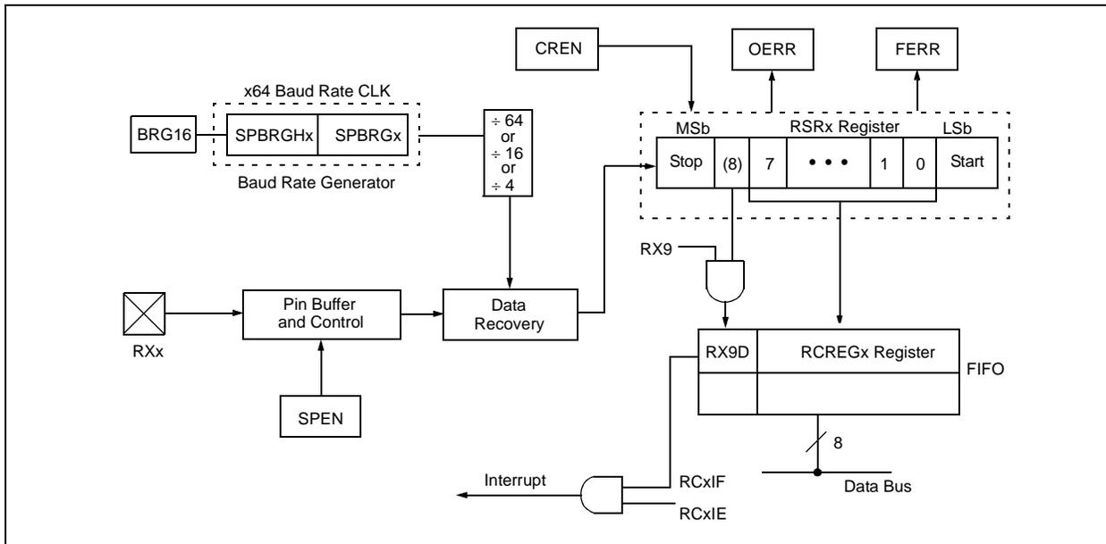
**FIGURE 20-7: ASYNCHRONOUS RECEPTION**
