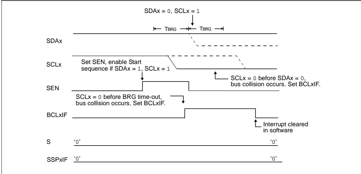
**FIGURE 19-28: BRG RESET DUE TO  $SDAx$  ARBITRATION DURING START CONDITION**
