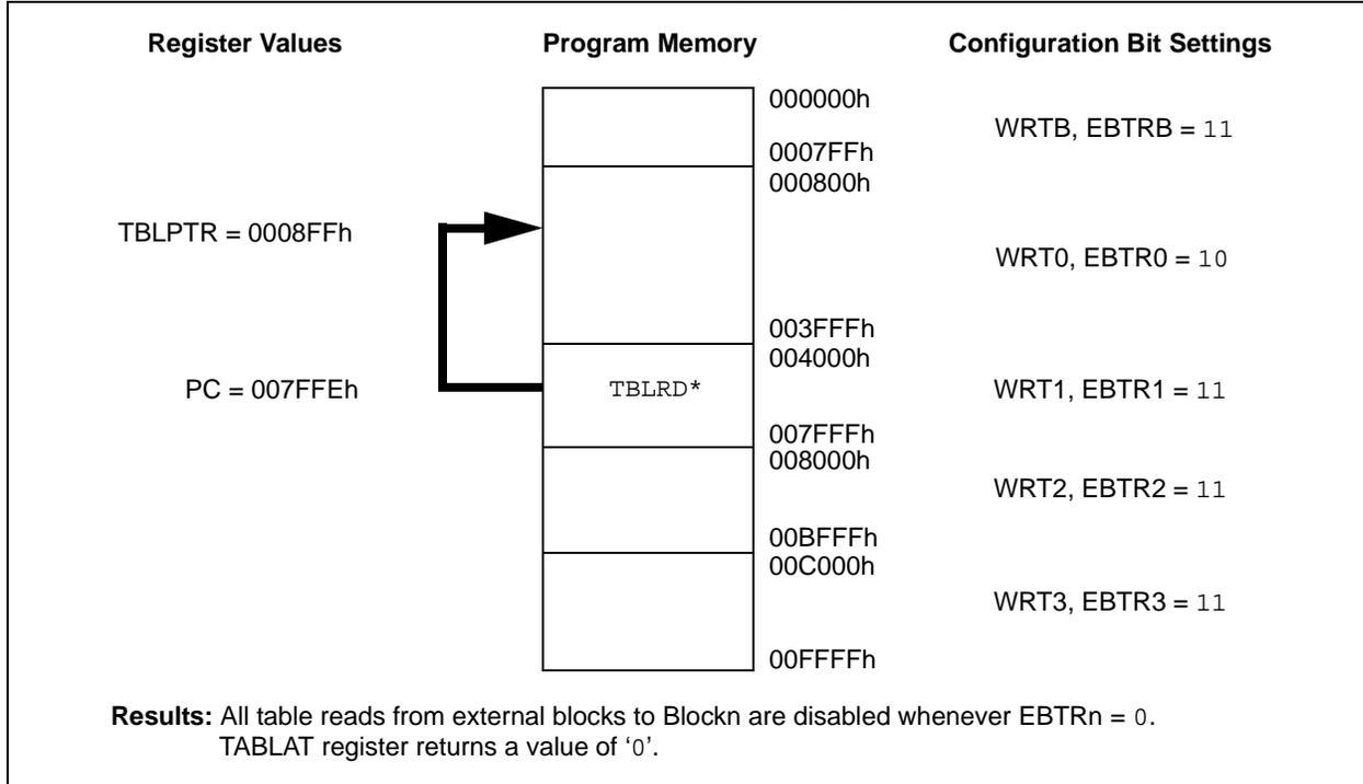
**FIGURE 25-8: EXTERNAL BLOCK TABLE READ (EBTRn) ALLOWED**
