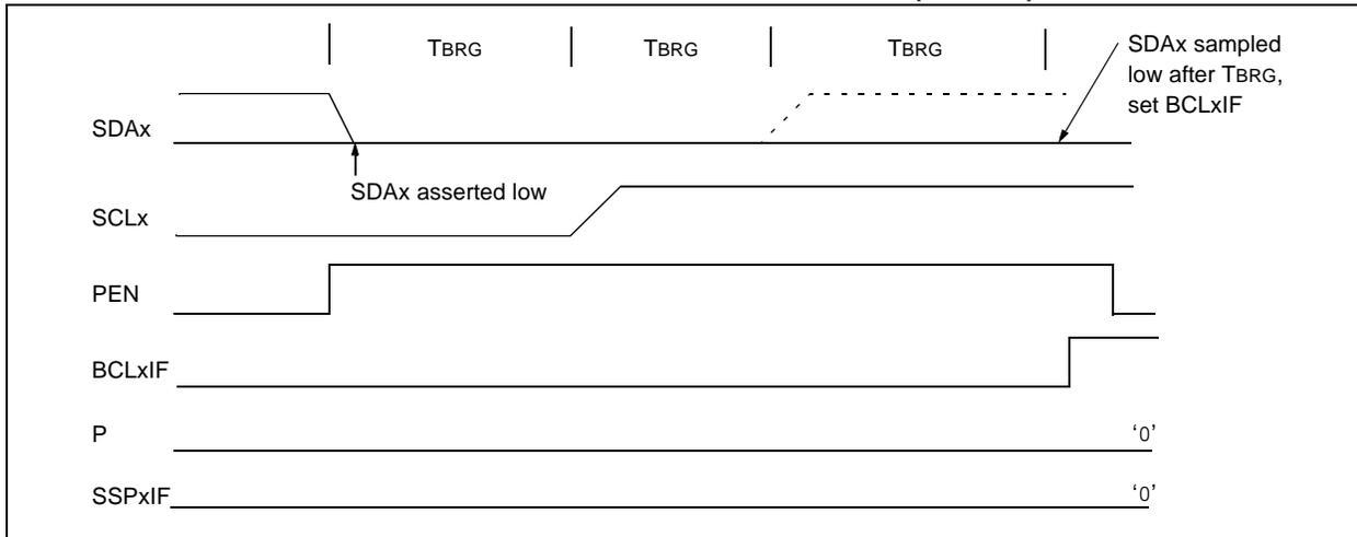
**FIGURE 19-32: BUS COLLISION DURING A STOP CONDITION (CASE 2)**
