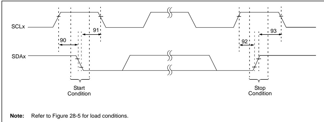
**TABLE 28-20: I<sup>2</sup>C™ BUS START/STOP BITS REQUIREMENTS (SLAVE MODE)**
