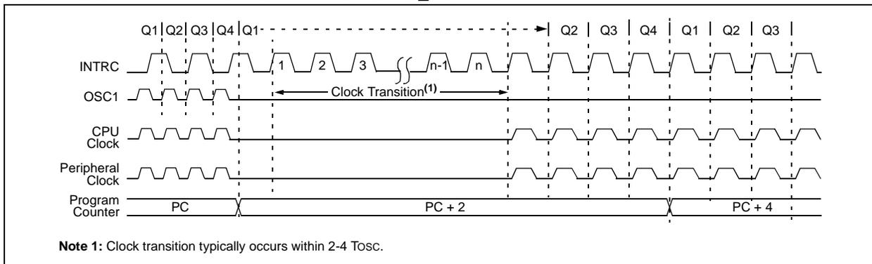
**FIGURE 3-4: TRANSITION TIMING FROM RC\_RUN MODE TO PRI\_RUN MODE**
