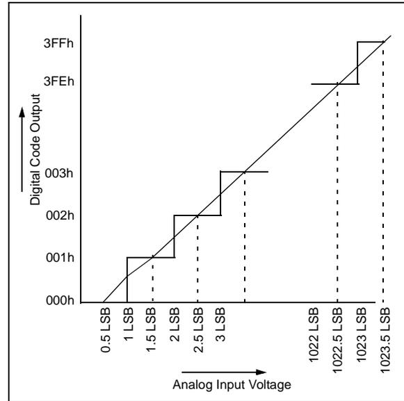
**FIGURE 21-3: ANALOG INPUT MODEL**
