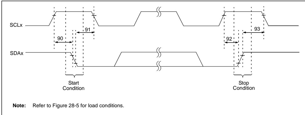
**TABLE 28-22: MASTER SSP I<sup>2</sup>C™ BUS START/STOP BITS REQUIREMENTS**
