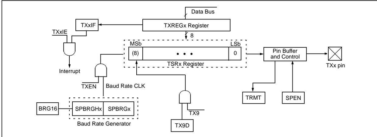
**FIGURE 20-4: ASYNCHRONOUS TRANSMISSION**
