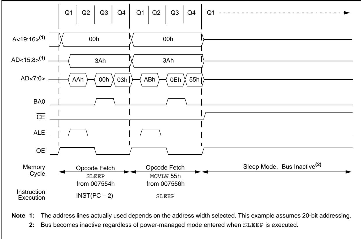
**FIGURE 7-11: TYPICAL OPCODE FETCH, 8-BIT MODE**
