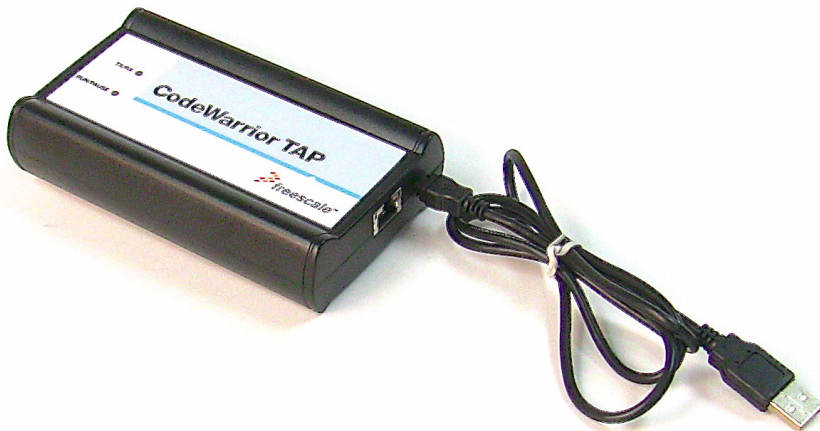
Figure 2.3 CodeWarrior TAP Probe with USB Cable Attached
