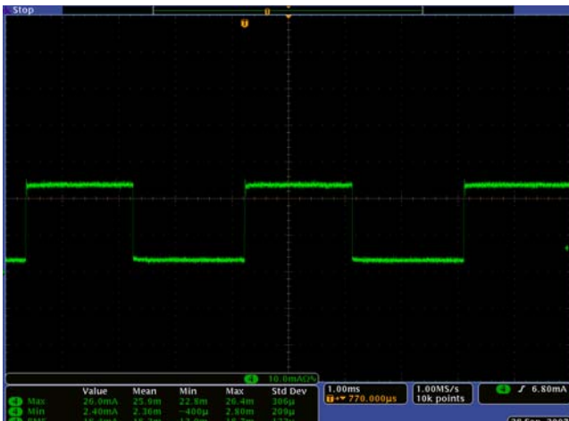
FIGURE 13. I_{LED} AT 50% PWM DIMMING
