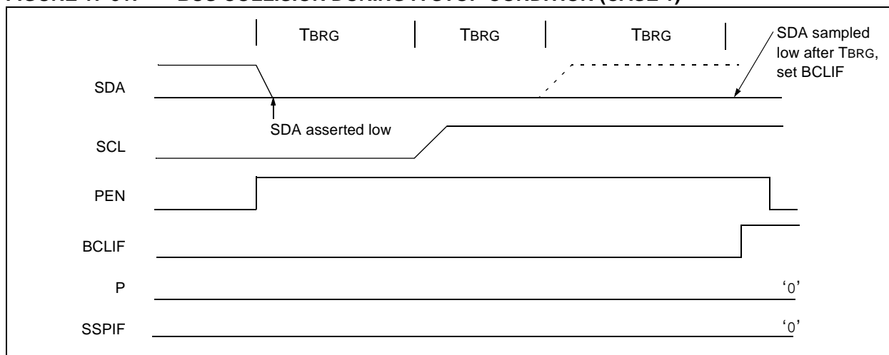
FIGURE 17-31: BUS COLLISION DURING A STOP CONDITION (CASE 1)
