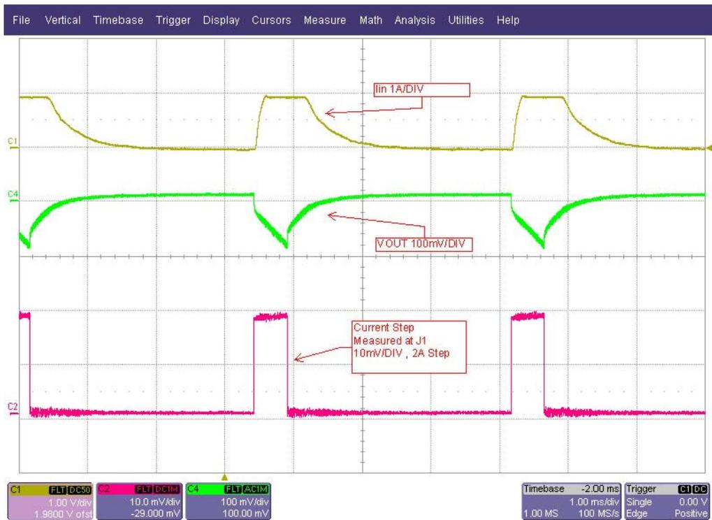
Figure 3. Step Load Response
