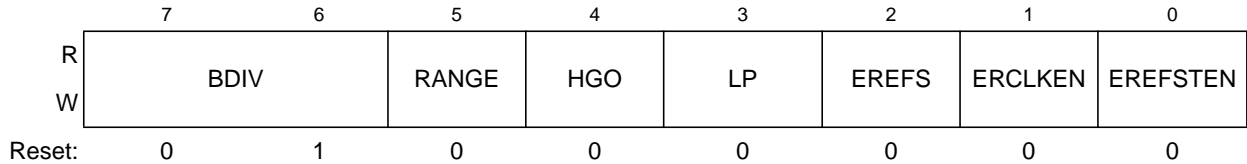
Figure 8-4. MCG Control Register 2 (MCGC2)
