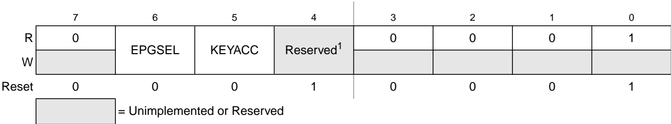
Figure 4-7. Flash Configuration Register (FCNFG)
