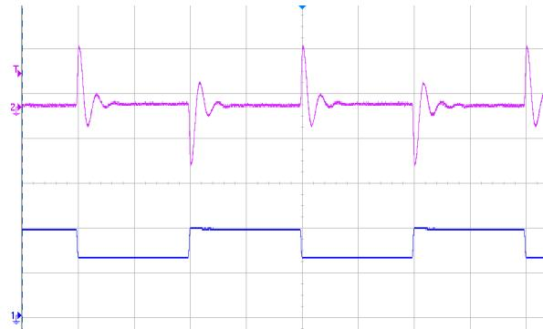
Figure 5 Dynamic response for 25% load step (50% ~ 75% ~ 50%) and 1A/ $\mu$ s slew rate, (2ms/div), see Figure 10 for test configuration; CH2-output voltage (200mV/div); CH1-output current (10A/div)
