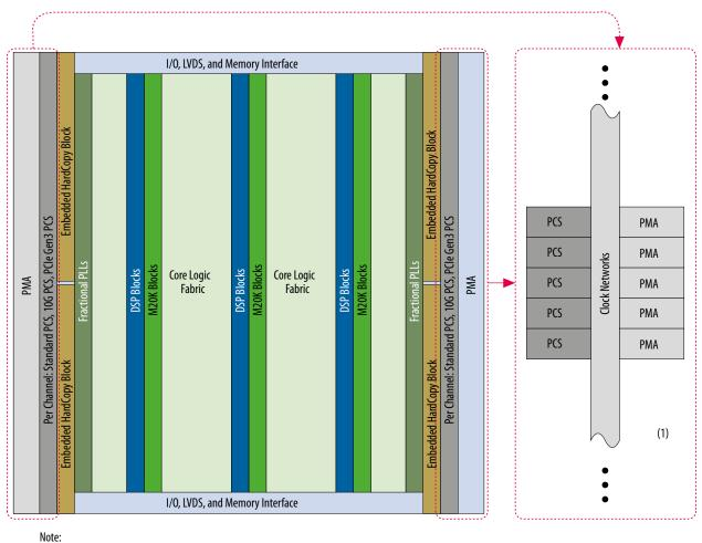
(1) You can use the unused transceiver channels as additional transceiver transmitter PLLs.
