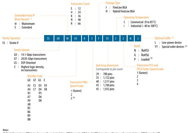
(1) Stratix V mainstream "M" devices have exactly one instantiation of PCI Express hard IP. Extended "E" devices have either two or four instantiations of PCI Express hard IP, depending on the device and package combination. For non-transceiver Stratix V devices, this character does not appear in the part number.
