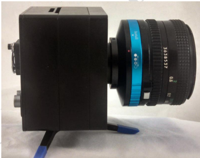
Figure 7 Compact Body Camera Option Shown with example lens and small tripod, side view
