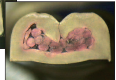
Visible Deformation of Outer Crimp Surface as a result of Indentation from Material Buildup on Crimper
