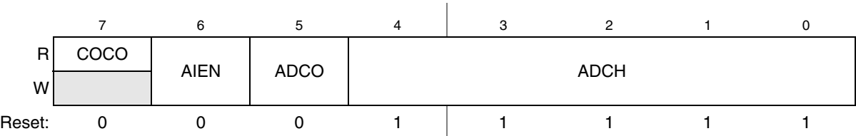
Figure 10-3. Status and Control Register (ADCSC1)
