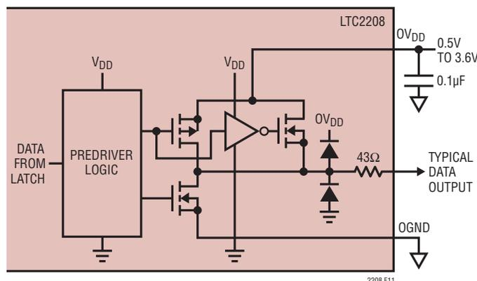
Figure 11. Equivalent Circuit for a Digital Output Buffer
