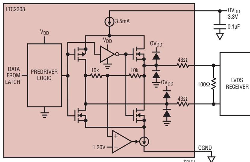
Figure 12. Equivalent Output Buffer in LVDS Mode
