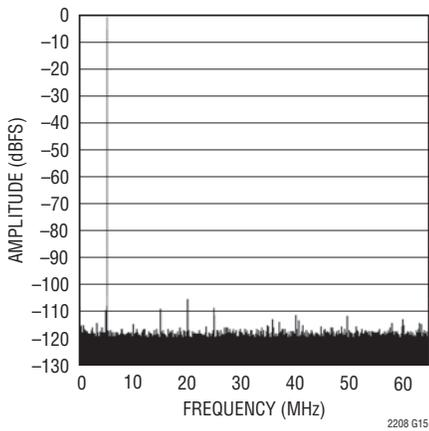
**64k Point FFT,  $f_{IN} = 15.1\text{MHz}$ , -1dBFS, PGA = 0**
