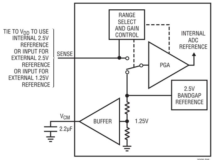
**Figure 6. Reference Circuit**
