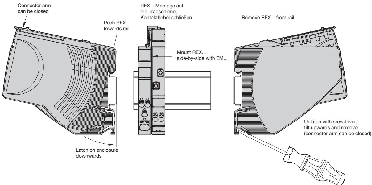
**Application example: REX... Replacement or disassembly**
