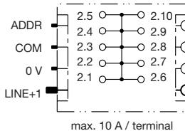
**PM12-T02-00-LOAD-20A potential module – LOAD
